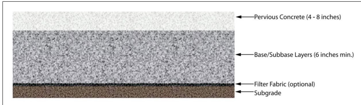
Figure 19 Typical pervious concrete pavement cross section.
