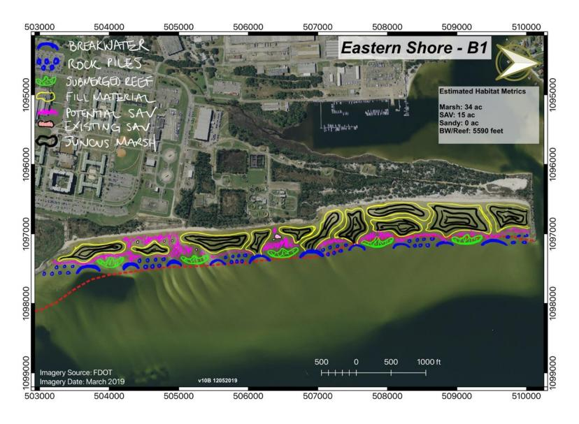
Figure 9: Preliminary conceptual design (B1) for the Eastern Shore (Site B).
