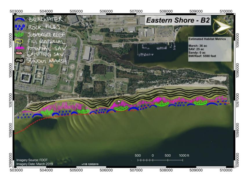
Figure 10: Preliminary conceptual design (B2) for the Eastern Shore (Site B).
