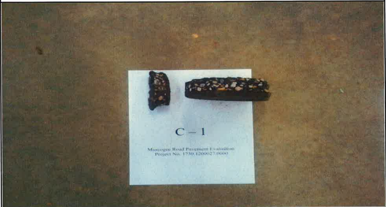
Photo 2: Pavement core C - 1. Unable to extract full core depth of 6 inches.
