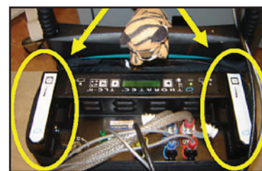
Batteries loaded into battery slots on TLC-II Driver
