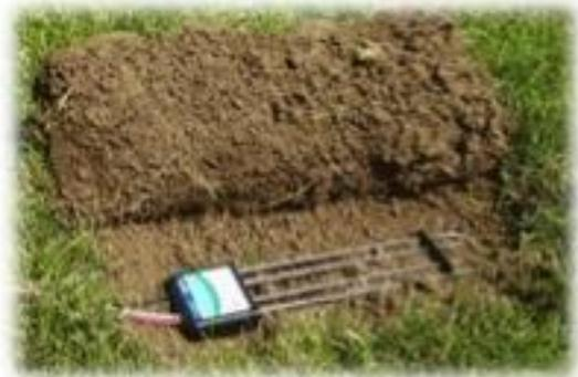
sensors (SMS). When using soil moisture sensors, the run time for each irrigation zone can be divided into several short cycles, allowing the moisture level to be checked between cycles to optimize the amount of water delivered
