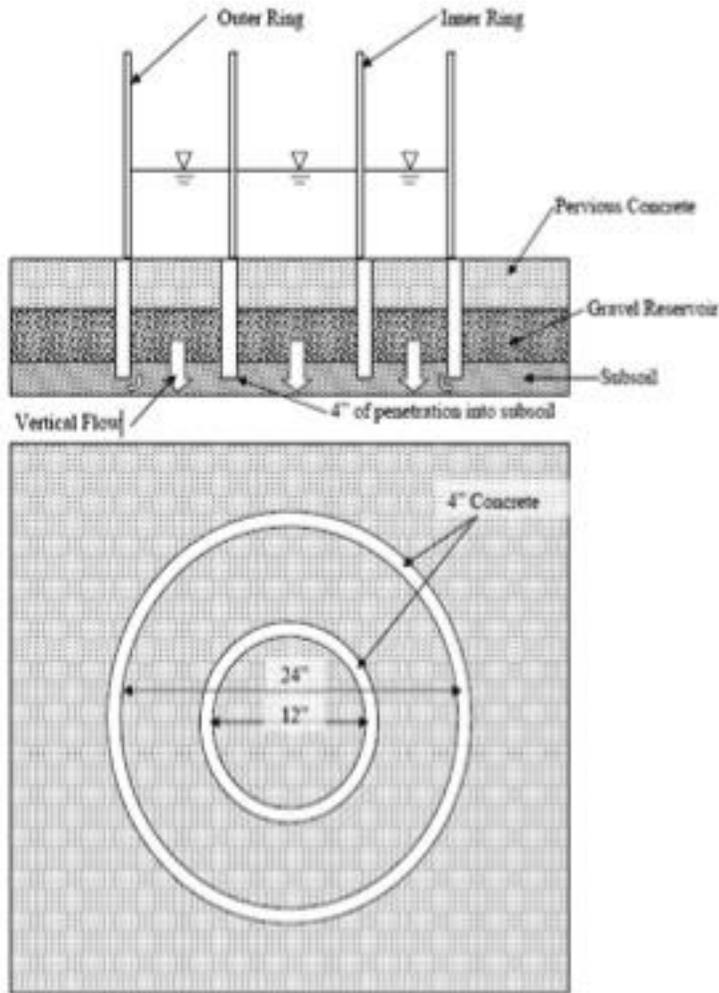
Figure 42: Design profile for Embedded Infiltrometer installation
