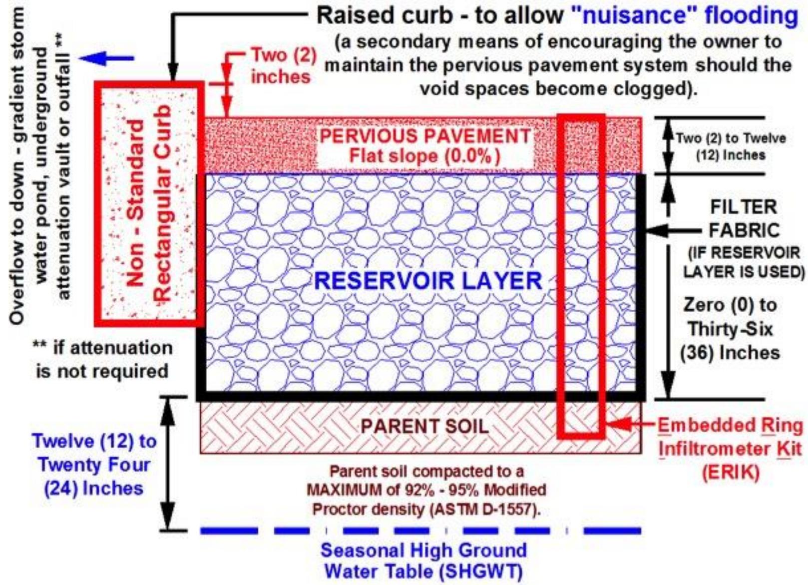
**Raised curb - to allow "nuisance" flooding**
