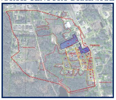
Acquisition of Wetland real estate to be preserved as mitigation as required by the Corps of Engineers for permitting the North Century Drainage Project that includes a stormwater retention/treatment system to ensure U.S. 29 remains open (unflooded) as a hurricane evacuation route and to improve water quality in the Escambia River System that flows into Escambia Bay, an impaired water body.
