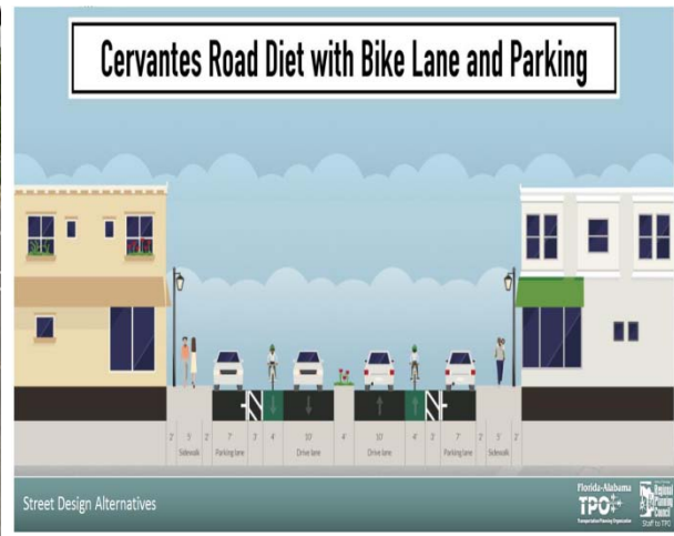
PHOTO SIMULATION OF DESIRED IMPROVEMENTS FOR A PRIMARY COMMERCIAL CORRIDOR, WEST CERVANTES STREET COORIDOR MANAGEMENT PLAN.
