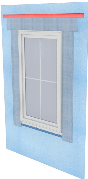
Figure 4. Example flashing details for a flanged window installed over rigid foam insulation sheathing installed as the WRB.
