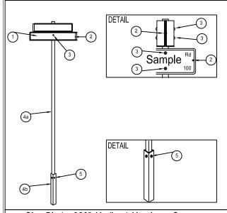
Install Street Name Signs on Corners Of Intersection so that they will be on the Far Right Side on the Intersection for Traffic on the Major Street in accordance with MUTCD Section 2D.38
