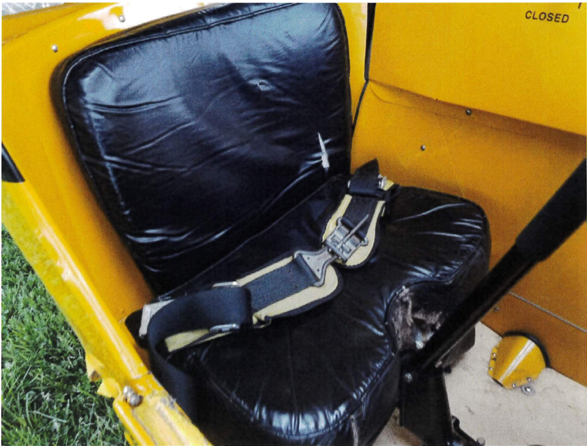
A simple lap belt holds the pilot into the airplane. The seatbelts are black with yellow padding.
